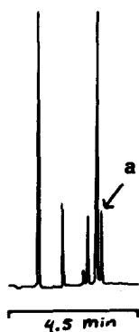
Fig. 5. Analysis of evening primrose oil on column B at 210°C. TCD temperature, 250°C. a = \gamma -linolenic acid.
